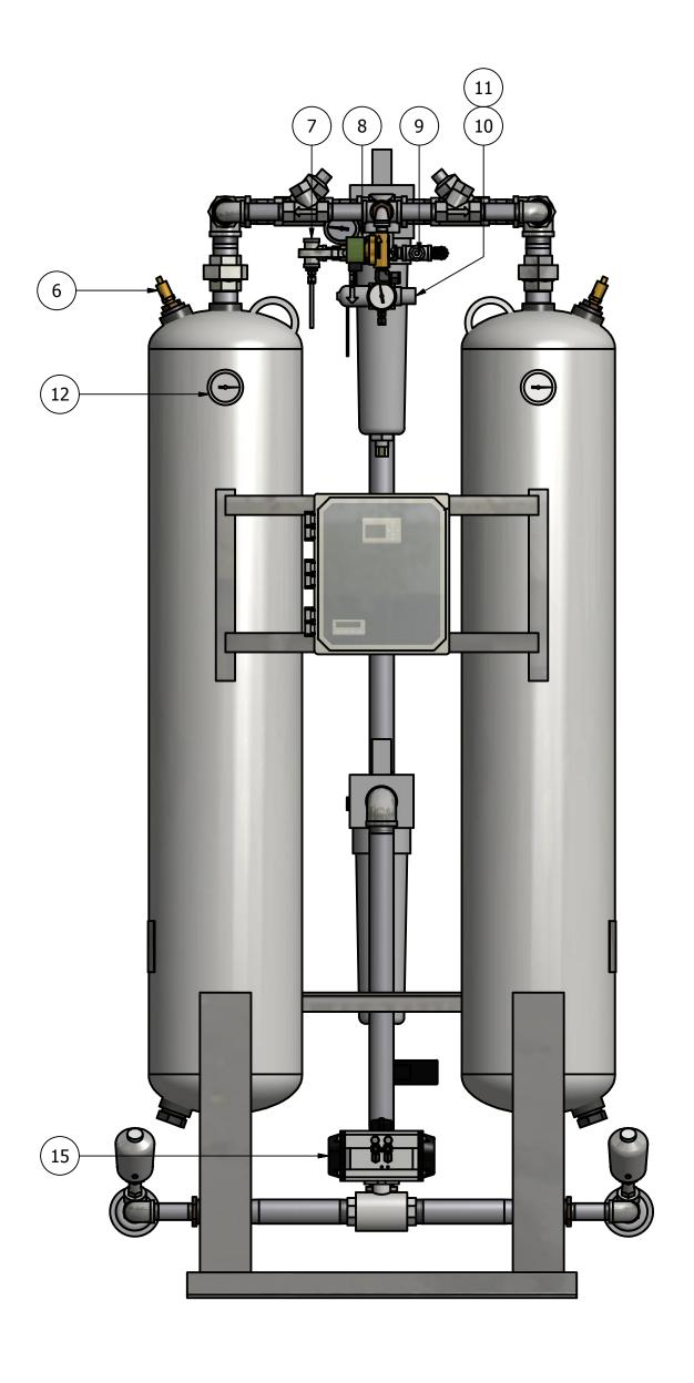
DESCRIPTION ITEM QTY CHECK VALVE, PURGE 2 PRESSURE REGULATOR, PURGE 2 PRESSURE GAUGE, PURGE 3 CHECK VALVE, OUTLET 4 PARTICULATE AFTER-FILTER 5 RELIEF VALVE, TANK 6 DEW POINT MONITOR (OPTIONAL) SOLENOID VALVE, REPRESS 8 MOISTURE INDICATOR 9 1 10 PRESSURE REGULATOR, CONTROL PRESSURE GAUGE, CONTROL 11 12 PRESSURE GAUGE, TANK 13 COALESCER PRE-FILTER TIMED DRAIN 14 1 3 WAY BALL VALVE, INLET 15 ANGLE BODY VALVE, EXHAUST 16 MUFFLER, EXHAUST 17 MANUAL BALL VALVE, BYPASS 18 275 LBS DESICCANT
